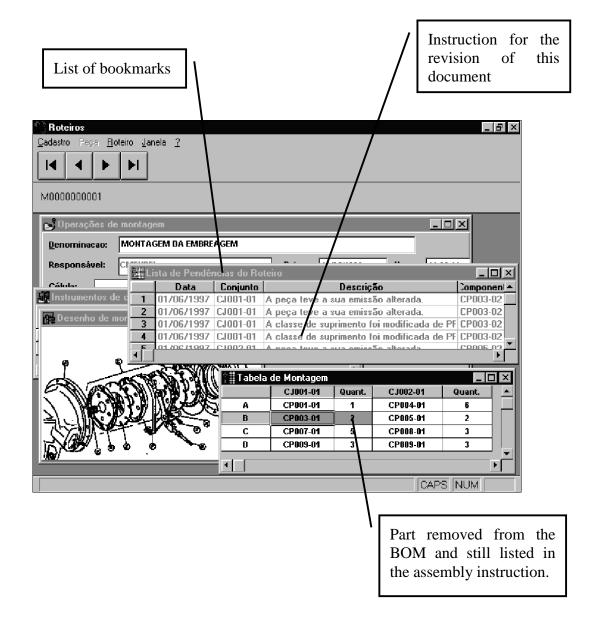
Figure 3: Control of inconsistencies in an assembly instruction
